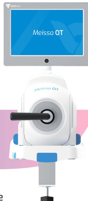
Meissa OT is an advanced robot designed for upper limb rehabilitation. It serves both as a training and assessment tool, utilizing a 4-channel EMG/EMS (Electromyography/Electrical Muscle Stimulation) system.
